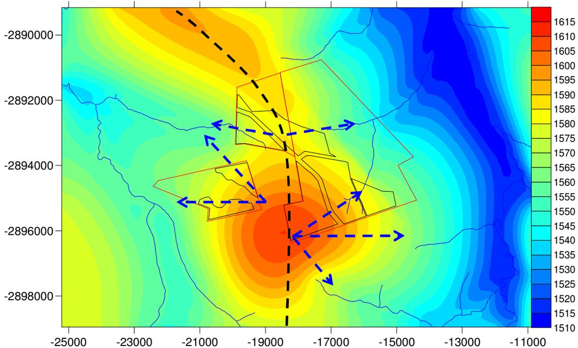
**Figure 1.3.1-3: Bayesian interpolated and steady state calibrated water level contour map for the proposed Stuart South Block model area**
