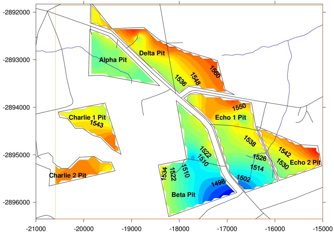
**Figure 1.3.1-4: Digital contour model of the base of the 2 Seam**
