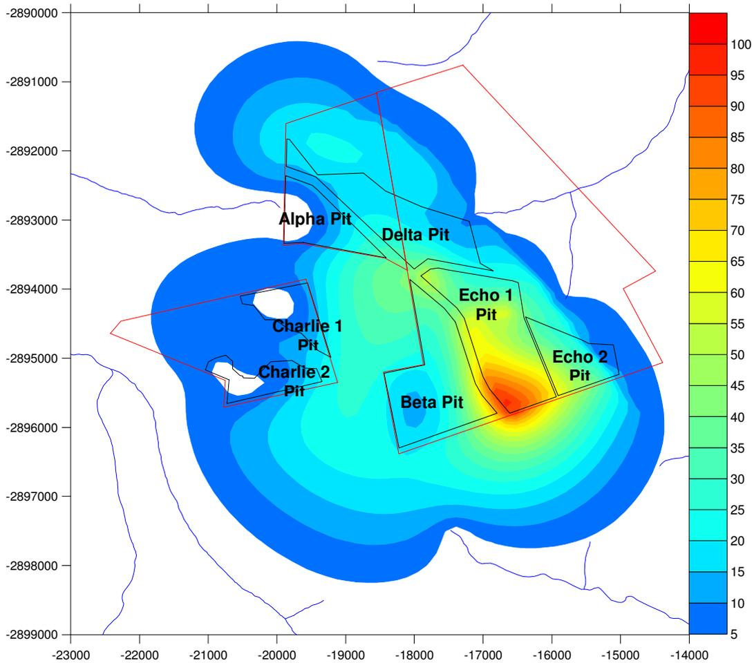
**Figure 3.3.1-2: Maximum water level impacts at mine closure**
