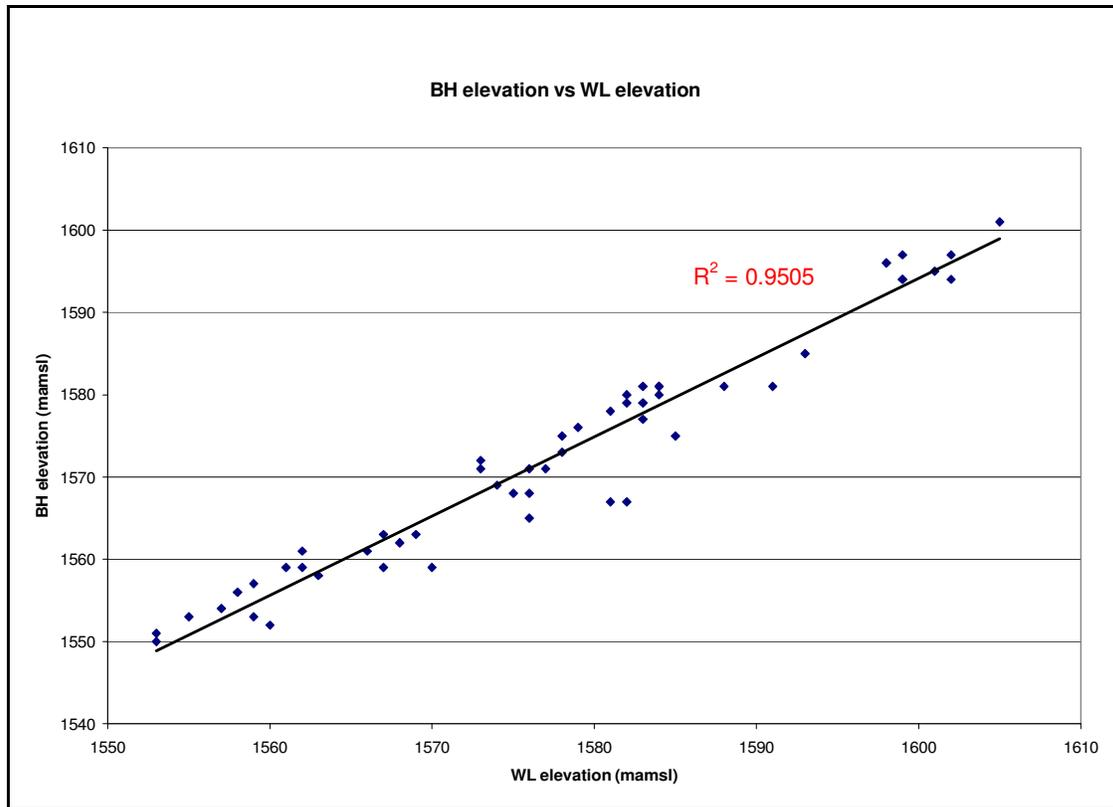
**Figure 1.3.1-2: Graph of borehole elevation versus water level elevation: Karoo Aquifer**
