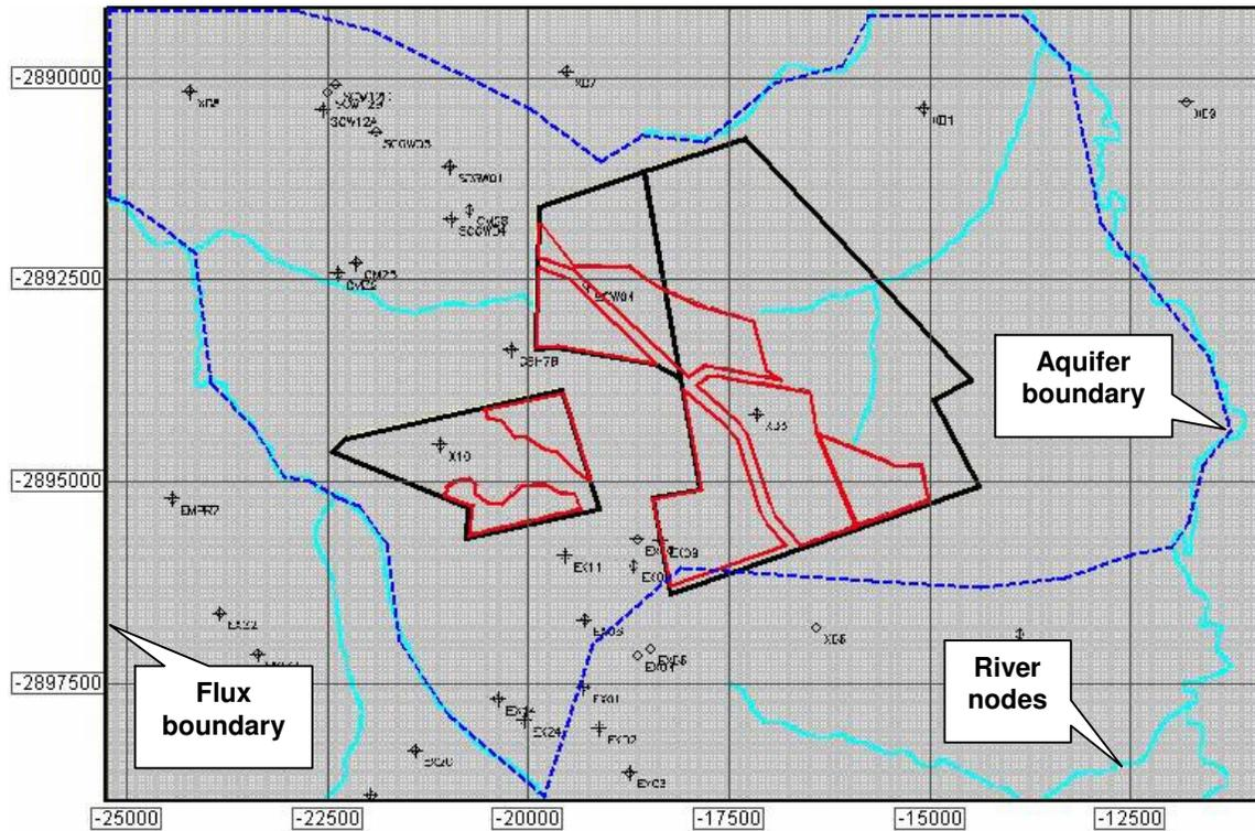
**Figure 1.2.2.4: Regional Stuart South Block model area with river nodes and flux boundaries**
