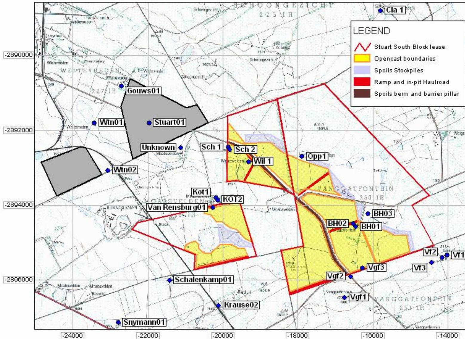
Figure 1.2.1: Boreholes recorded during the CSSS hydrocensus survey of the area
