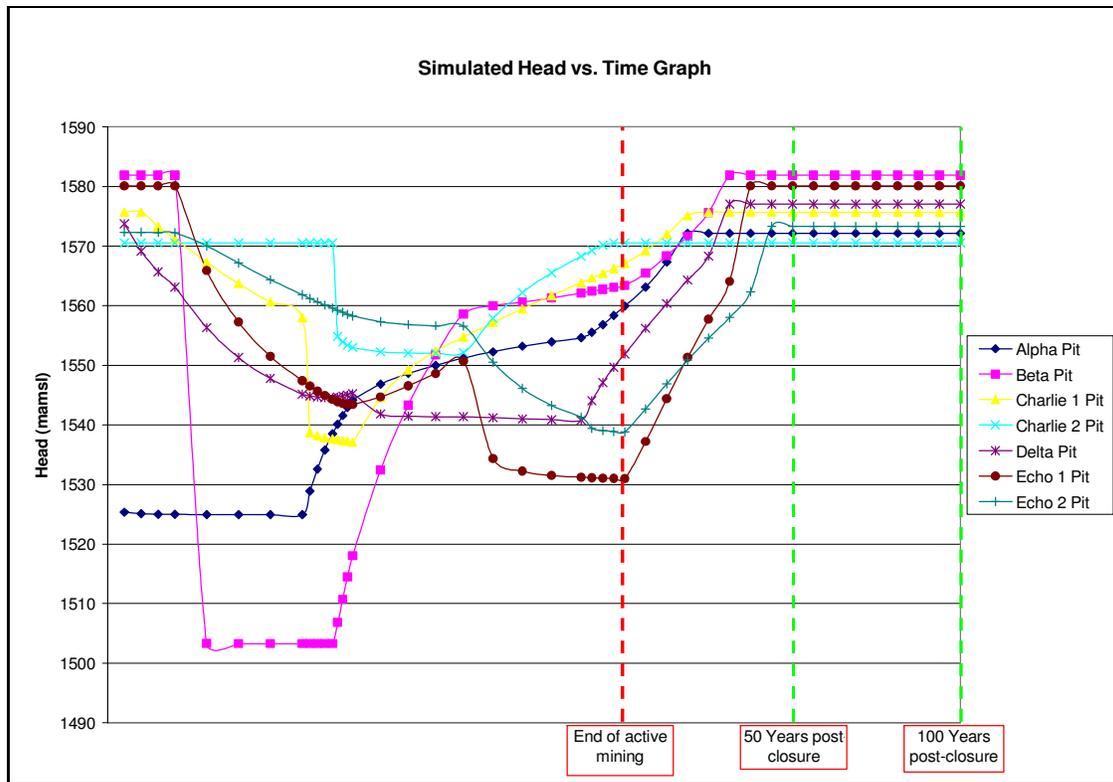
**Figure 3.3.1-3: Simulated head vs. time curves**
