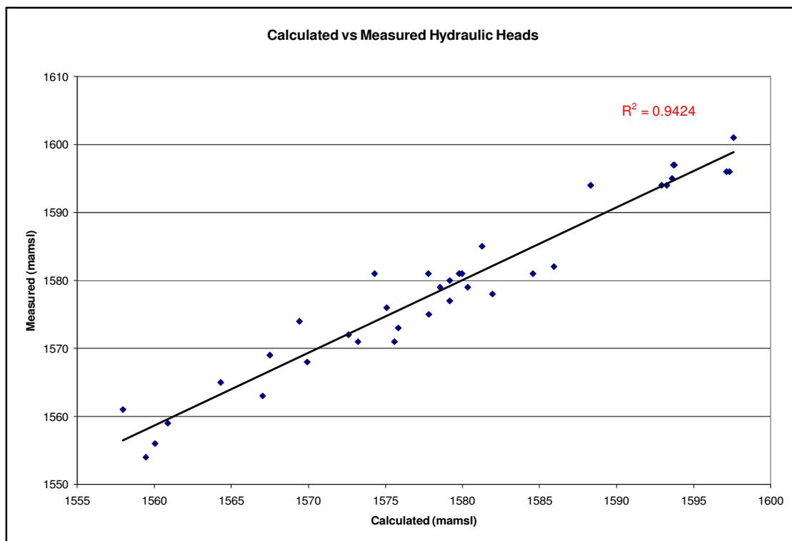
**Figure 3.3.1-1: Calculated vs. observed hydraulic heads**
