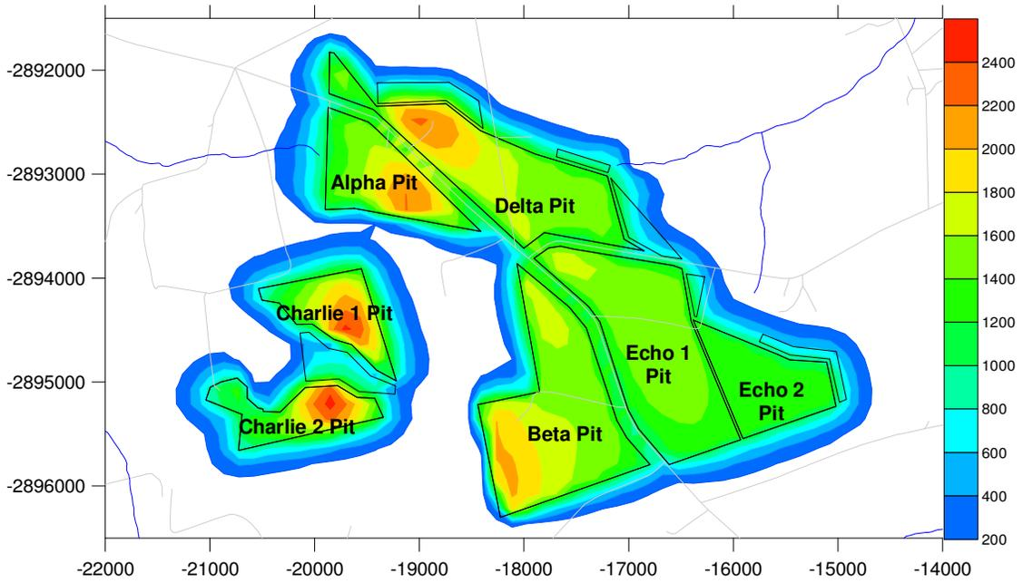
Figure 3.3.2-1: Simulated TDS source concentration contours 50 years post closure
